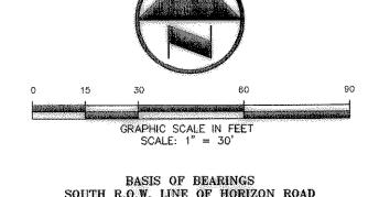
SOUTH R.O.W. LINE OF HORIZON ROAD S 45°37'17" E AS SHOWN ON PLAT HORIZON RIDGE ADDITION (CABINET E, PAGE 117, M.R.R.C.T.)
