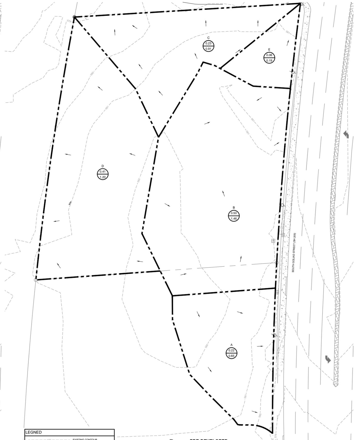
**POST-DEVELOPED RUNOFF CALCULATIONS - RATIONAL METHOD**
