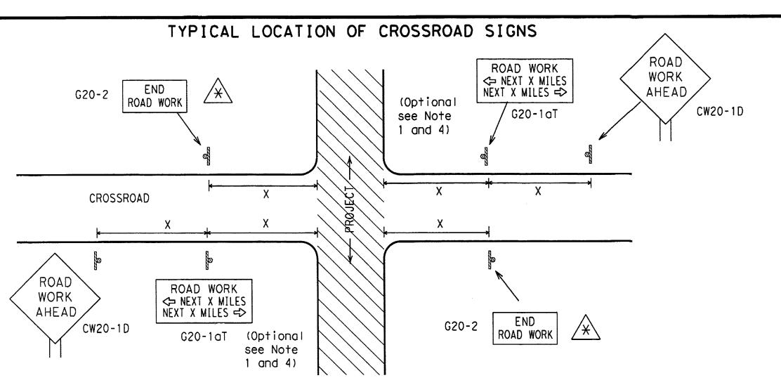
May be mounted on back of "ROAD WORK AHEAD" (CW20-1D) sign with approval of Engineer. (See note 2 below)
