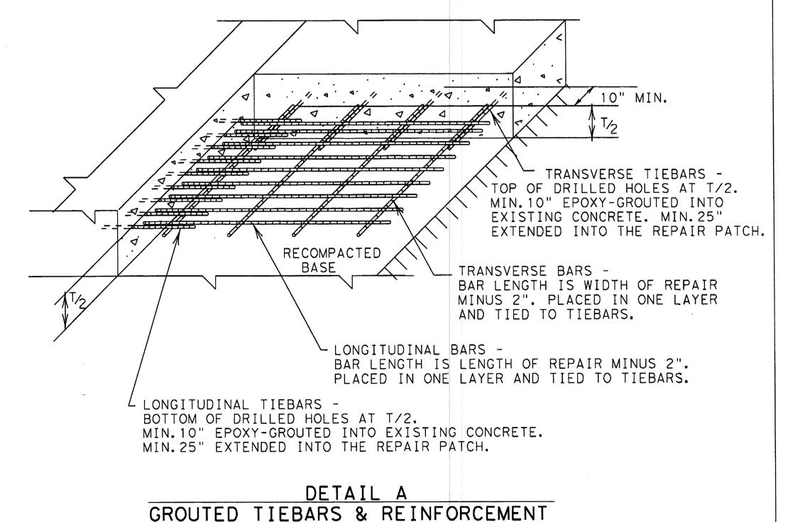
FULL-DEPTH REPAIR OF CRCP, JRCP, AND CPCD
