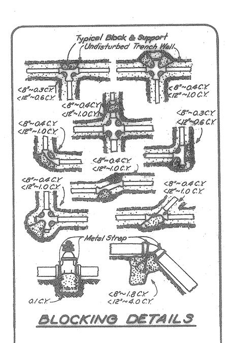
CONCRETE FOR BLOCKING SHALL HAVE A COMPRESSIVE STRENGTH OF NOT LESS THAN 2500 P.S.I. AT 28 DAYS. BLOCKING SHALL BE PLACED AGAINST UNDISTURBED TRENCH WALL AND SHALL NOT COVER JOINT
