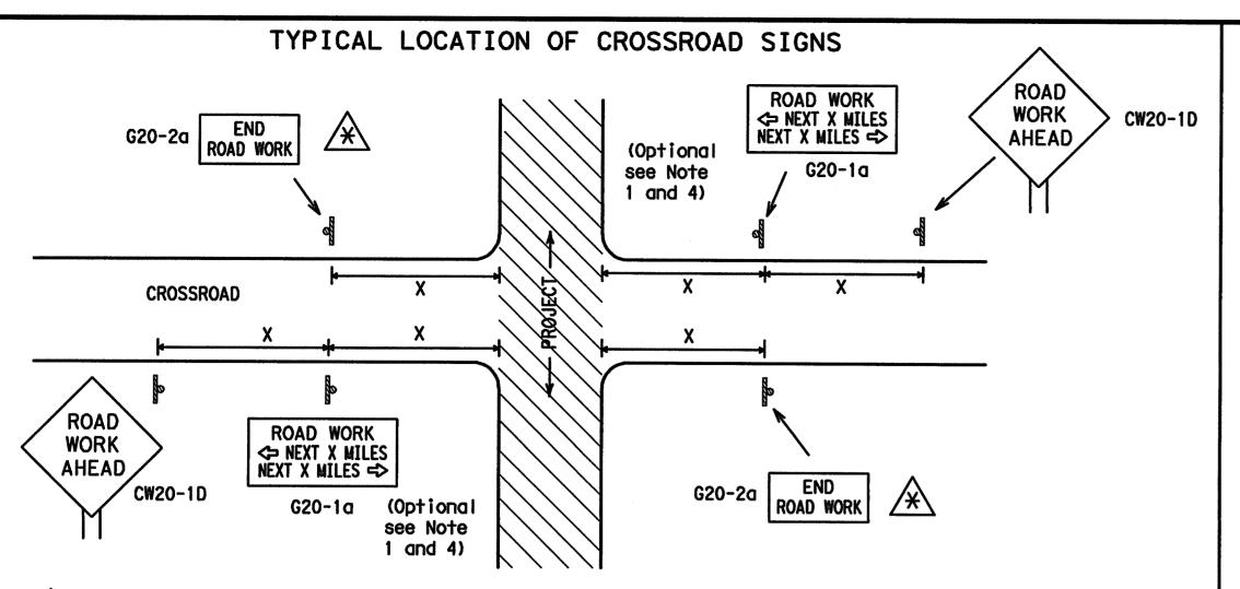
/X\ May be mounted on back of CW20-1D sign with approval of engineer. (See note 2 below)
