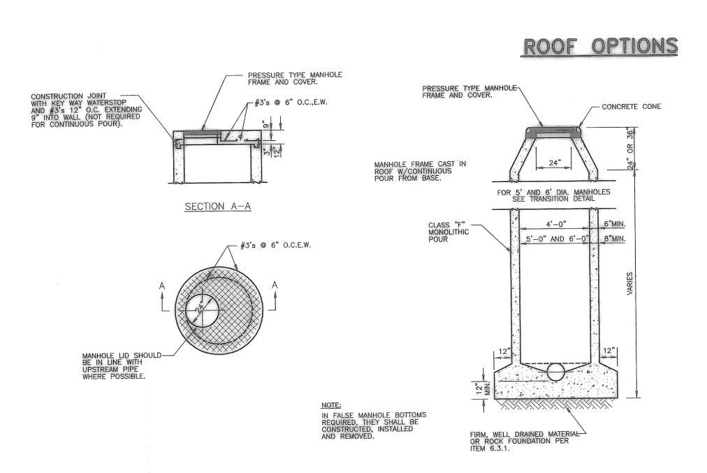
TYPE "S" MANHOLE (CAST IN PLACE)
