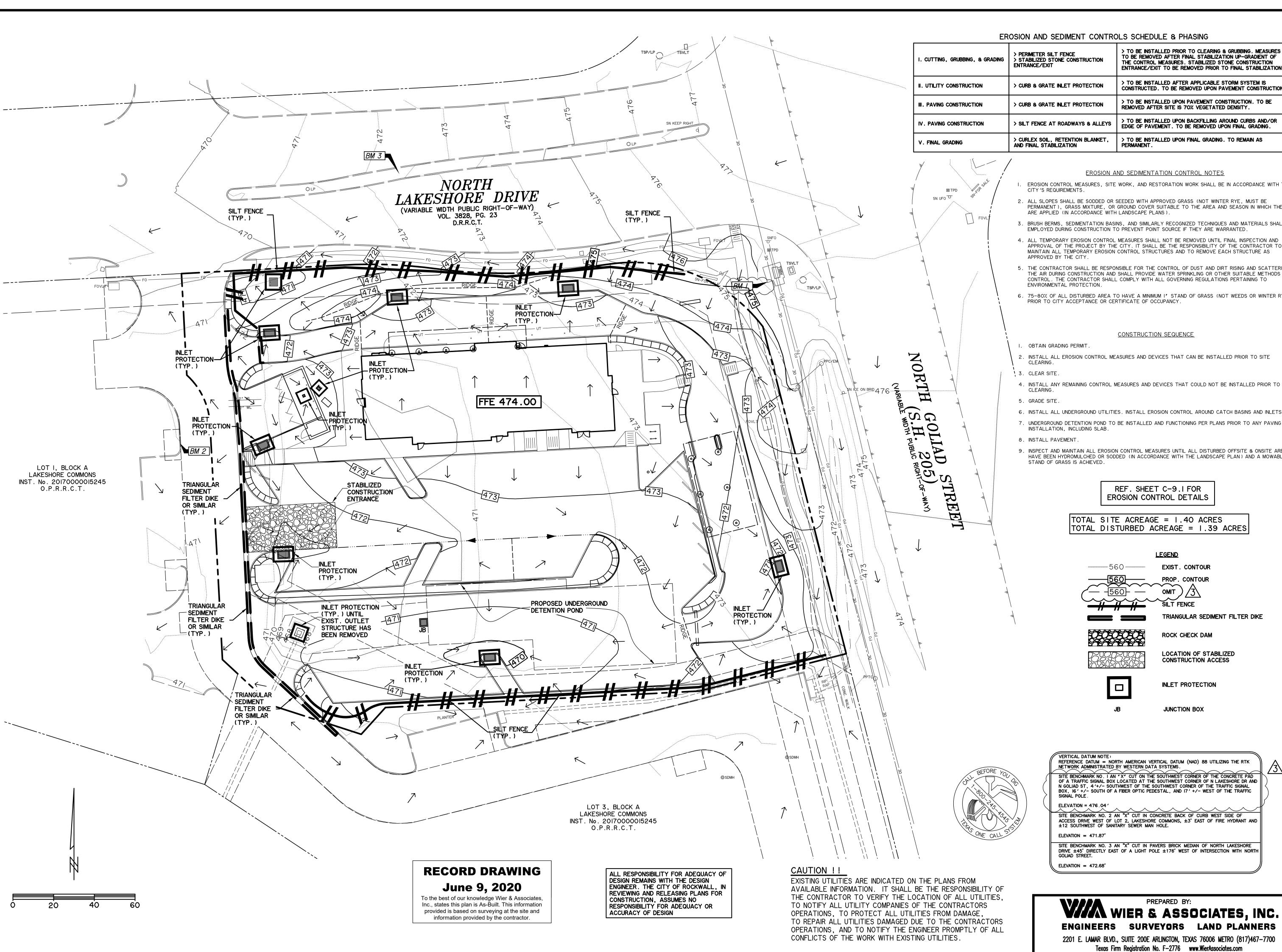
EROSION AND SEDIMENT CONTROLS SCHEDULE & PHASING
