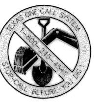
CONTRACTOR SHALL CALL 1-800-DIG-TESS FOR UTILITY LOCATIONS PRIOR TO ANY WORK IN EASEMENTS OR RIGHT-OF-WAY
