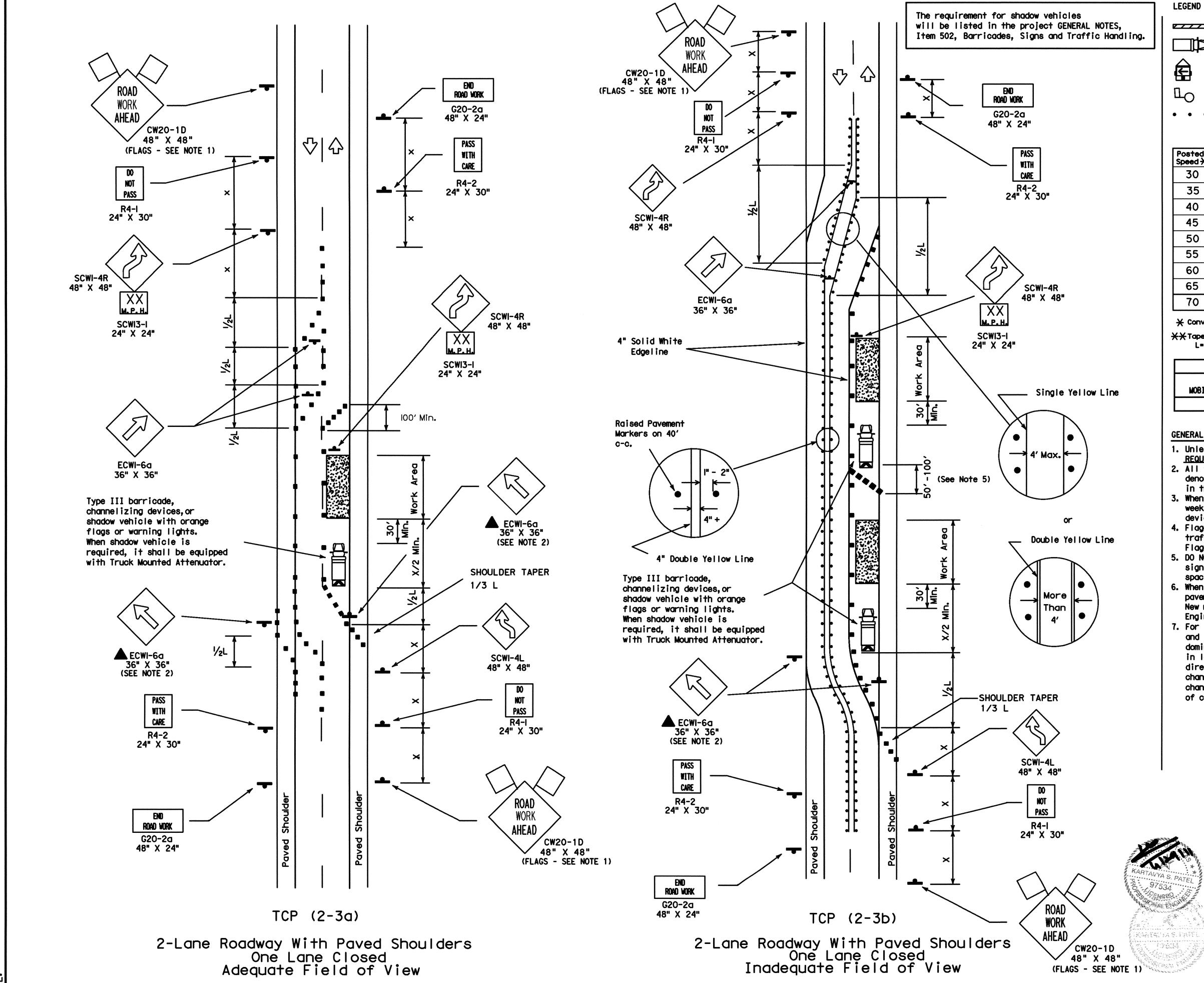
Type III Barricade ■ ■ Channelizing Devices
