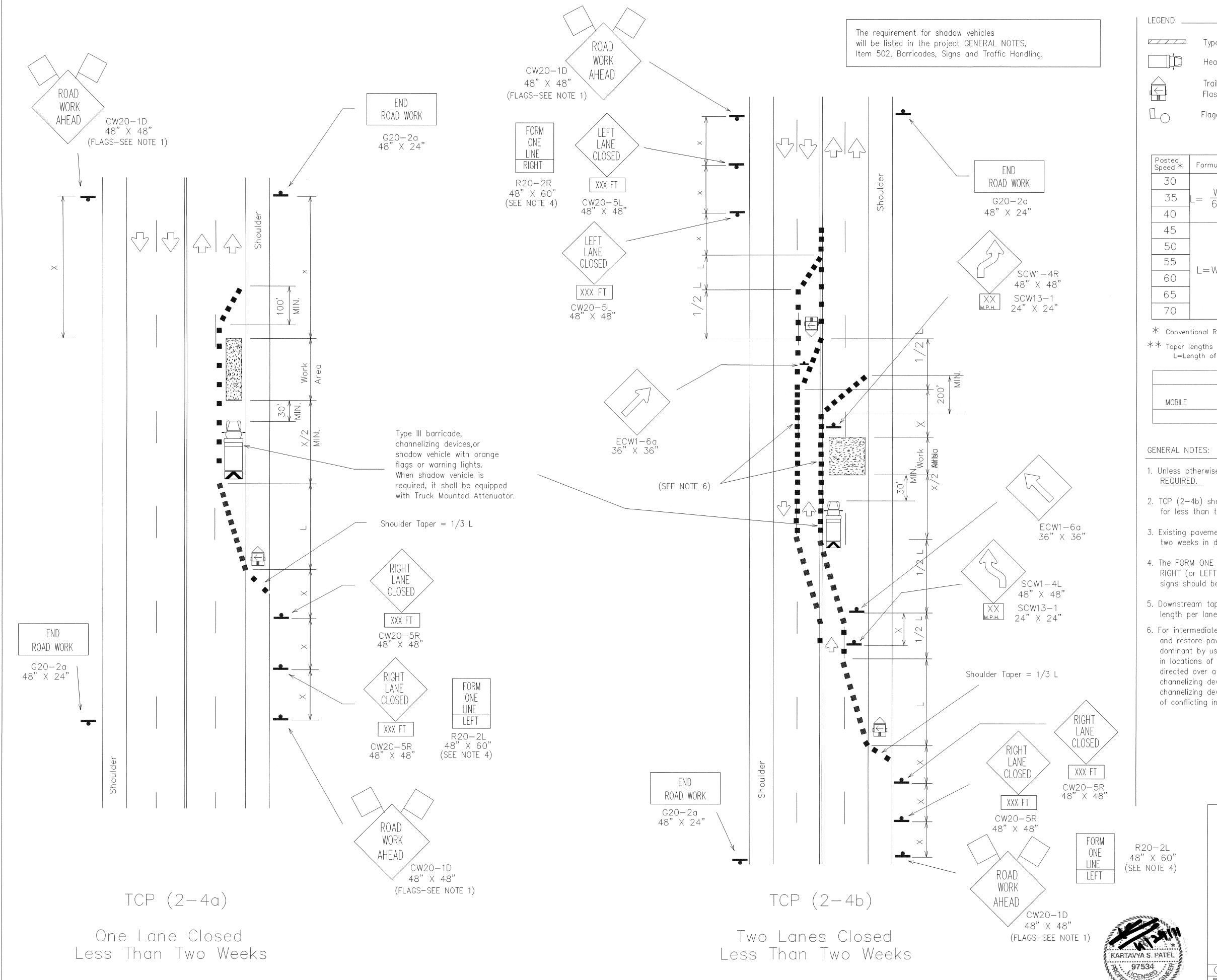
■ Channelizing Devices Flag Type III Barricade Truck Mounted Attenuator Heavy Work Vehicle Portable Changeable Trailer Mounted Message Sign Flashing Arrow Panel
