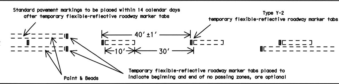
The traffic control devices detailed on this sheet will be furnished and erected as directed by the Engineer on sections of roadway where the surfacing operation has covered or obliterated existing pavement markings. These traffic control devices are to be used to supplement those required by BC Standards.
