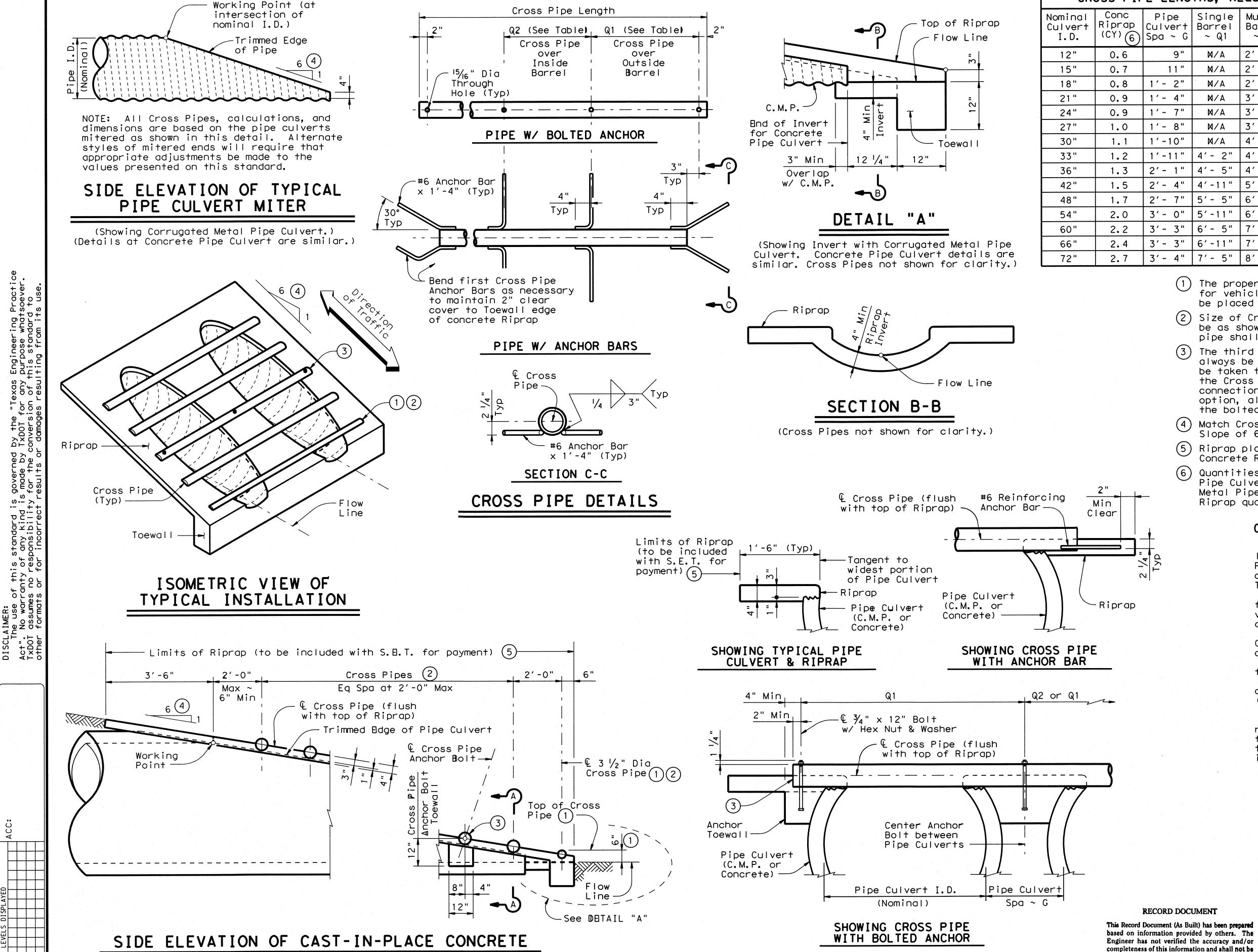
(Showing Concrete Pipe Culvert.) (Details at Corrugated Metal Pipe Culvert are similar.)
