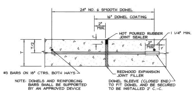
TRANSVERSE EXPANSION JOINT DETAIL NOTE: SPACE 60' O.C., LOCATE AT INTERSECTIONS
