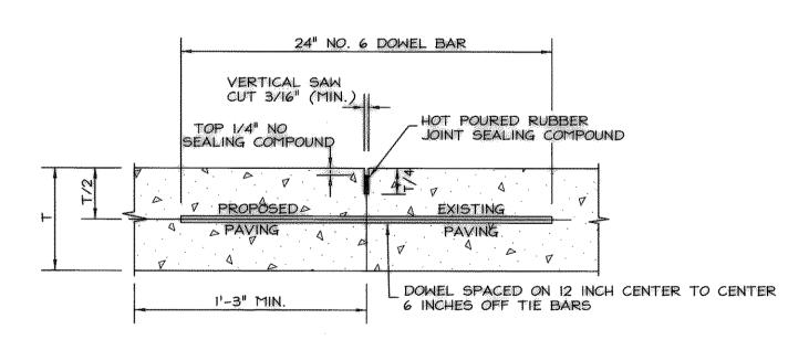
AT MARKINGS THE CONCRETE SHALL BE CUT I" DEEP, FOLLOWED BY GROOVING TOOL. STRENGTH SHALL BE 2500 p.s.i. WITH #3
