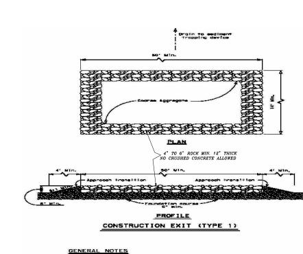
1. The length of the type 1 construction exit shall be as indicated on the picts, but not less than 50°.
