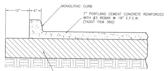
6" COMPACTED SUBRADE COMPACTED TO AT LEAST 95% OF MAXIMUM DRY DENSITY AT ±3% OF THE OPTIMUM MOISTURE PER ASTM D698
