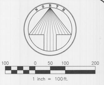
Basis of bearing: State Plane Coordinate System, North Texas Central Zone 4202, North American Datum of 1983. Adjustment Realization 2011.
