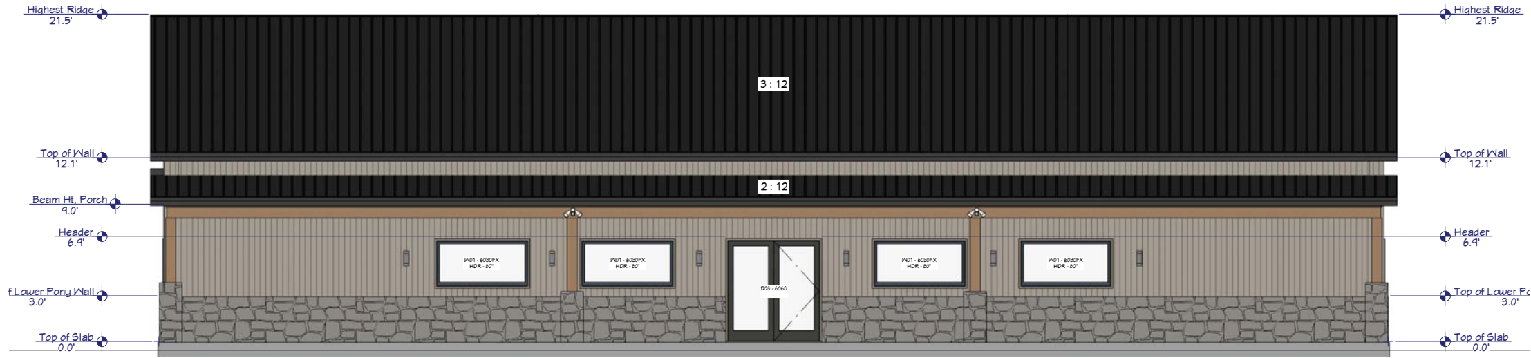
Exterior Elevation Front MATERIALS (EXCLUDES DOORS/WINDOWS & ROOF): R PANEL: 429 SF STONE PONY WALL: 245 SF (36%)
