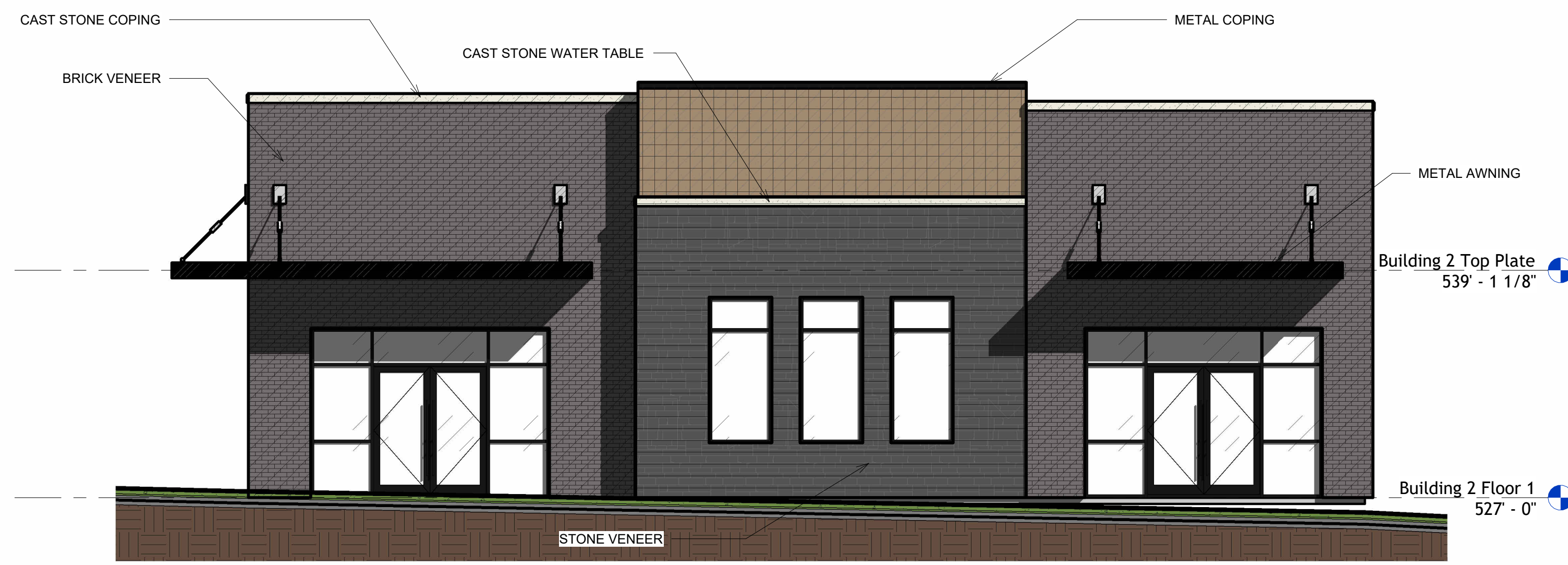
2 Building 2 North Elevation - Color 3/16" = 1'-0"
