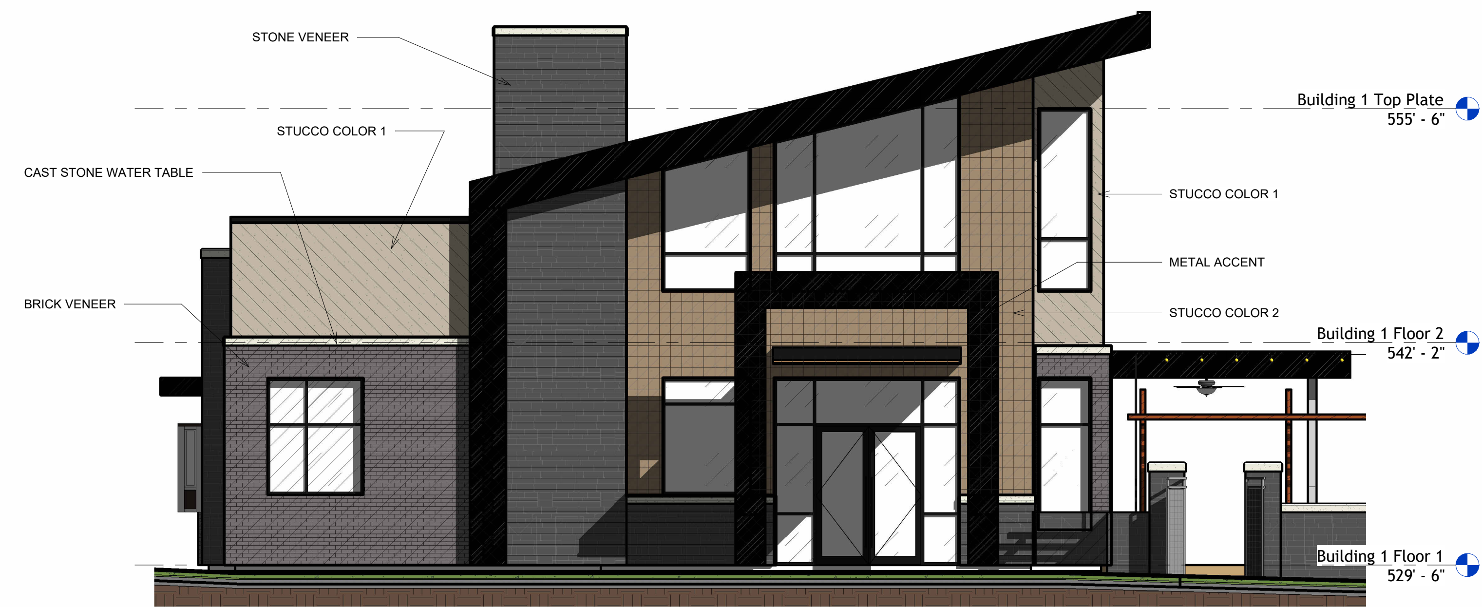
① Building 1 East Elevation - Color 3/16" = 1'-0"
