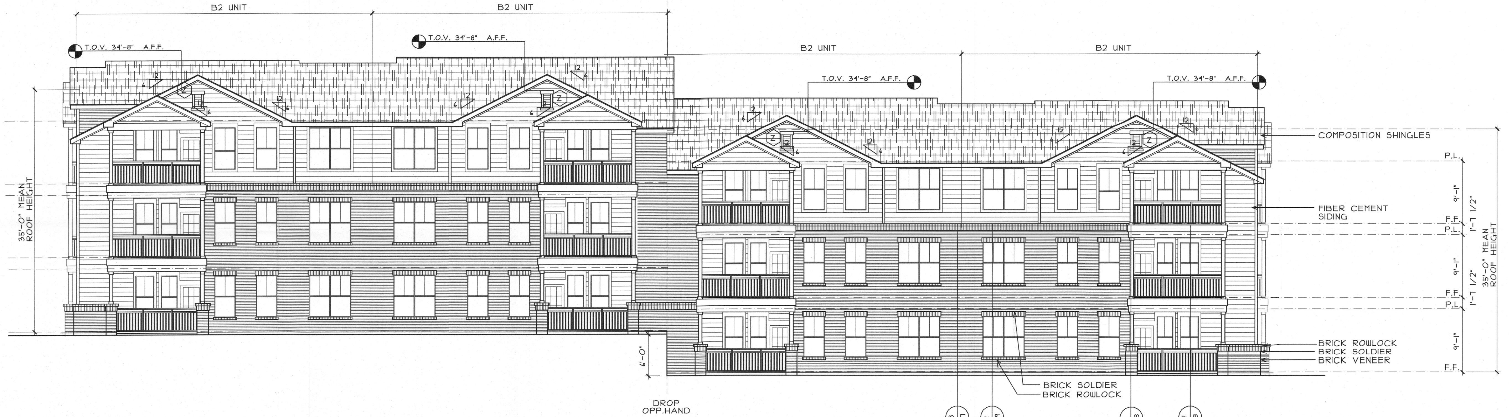
2 BUILDING TYPE 'A' - REAR ELEVATION SCALE 1/8"=1'-0"
