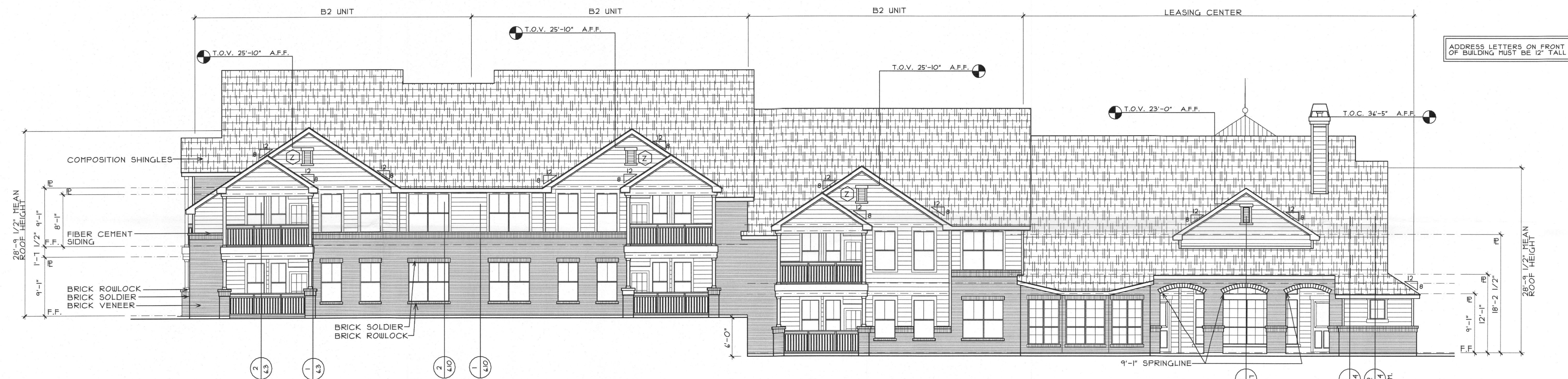
2 BUILDING TYPE 'A1' - REAR ELEVATION (BUILDING # 1) SCALE 1/8"=1'-0"
