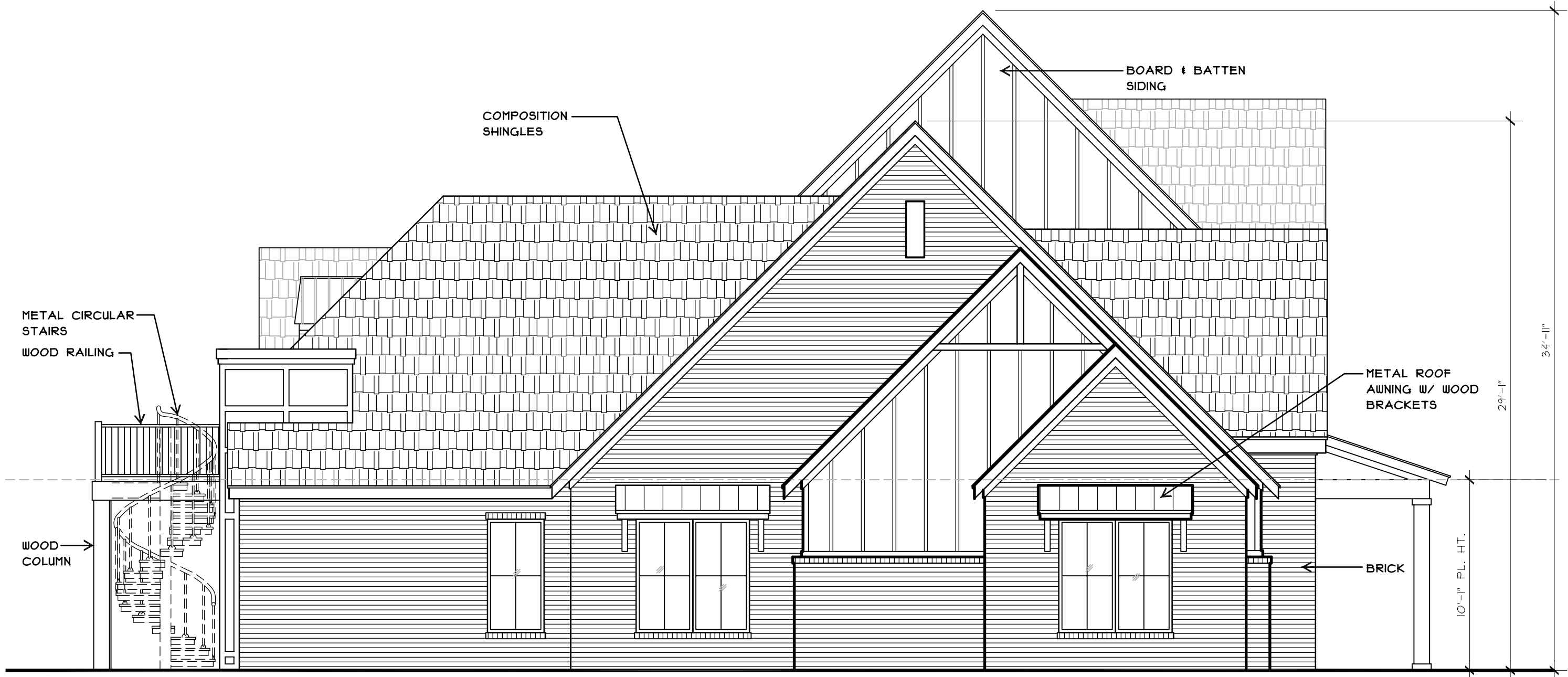
2 LEFT ELEVATION Scale: 3/32" = 1'-0"
