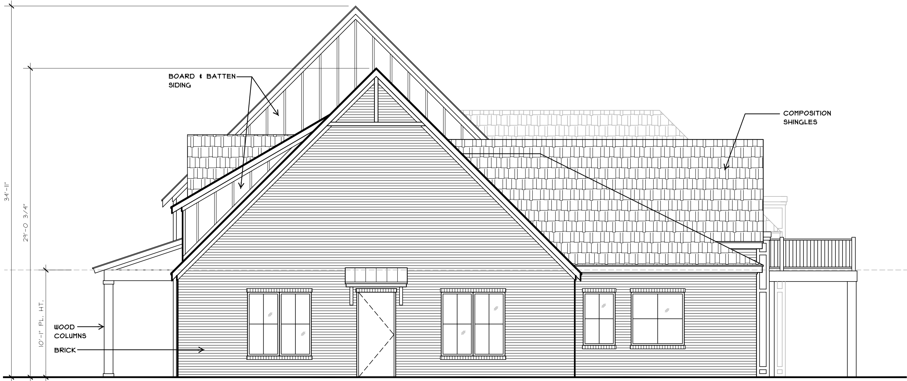
4 RIGHT ELEVATION Scale: 3/32" = 1'-0"
