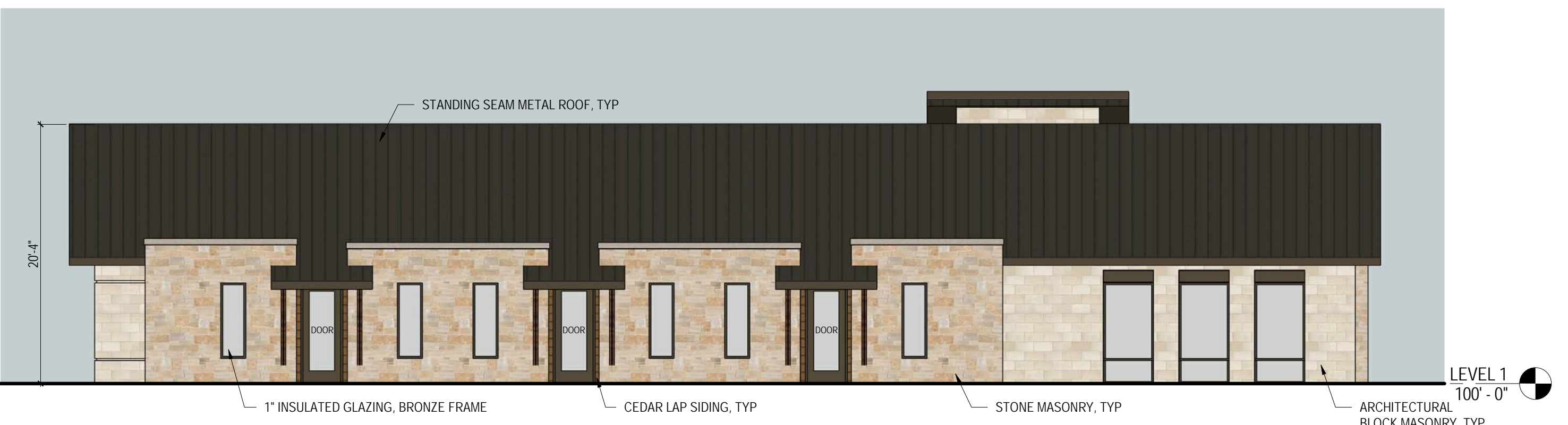
1 EXTERIOR ELEVATION - NORTHEAST
