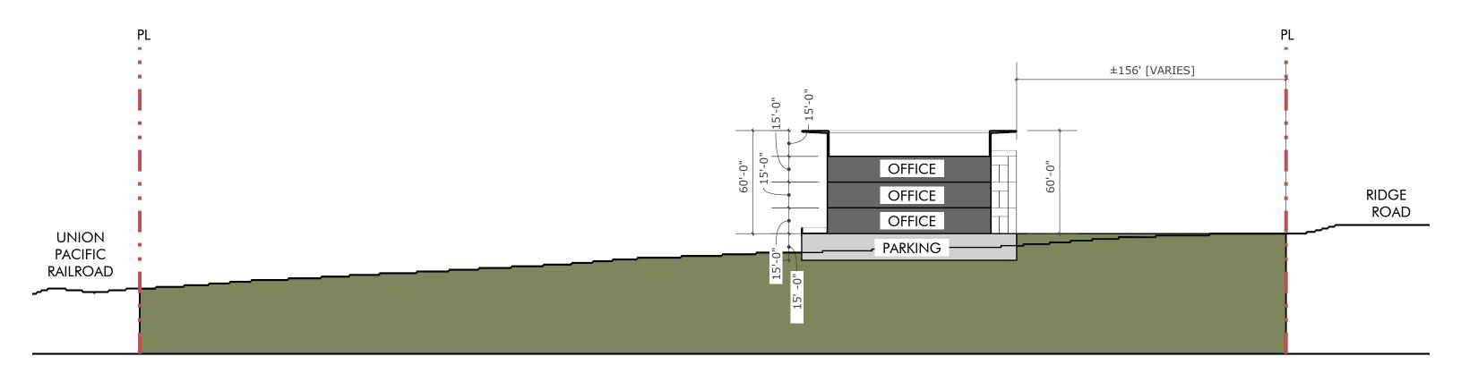
NOTE: FINISH FLOOR OF OFFICE WILL BE APPROXIMATELY 5'-7' FEET BELOW ADJACENT RIDGE ROAD ELEVATION AT MIDDLE OF SITE
