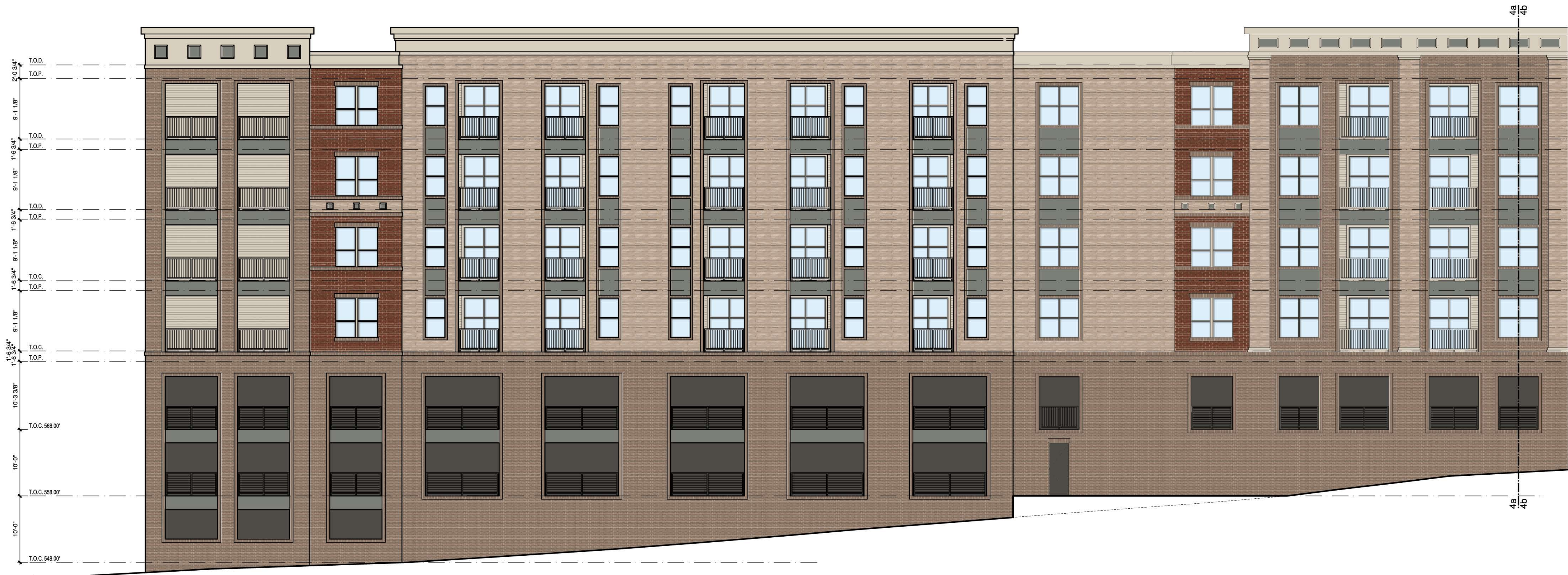
4a BUILDING - SOUTH ELEVATION (FIRST SOUTH STREET) SCALE: 1/8" = 1'-0"
