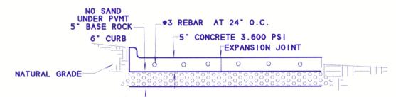
TYPICAL CONCRETE PAVEMENT CROSS SECTION
