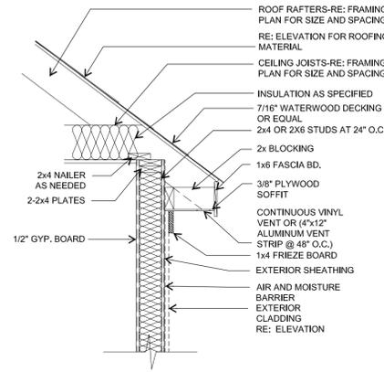
10 TYP. SOFFIT DETAIL
