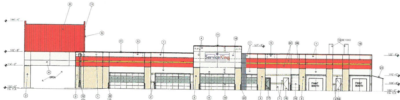
2 EAST ELEVATION SCALE: 3/32"=1'-0" 100% CMU BLOCK MASONRY 20% STUCCO 17% STUCCO 63% CMU BLOCK
