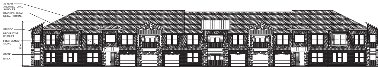
01 BUILDING F FRONT ELEVATION 3/32" = 1'-0"
