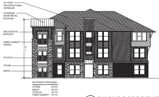
03 BUILDING G SIDE ELEVATION 3/32" = 1'-0"
