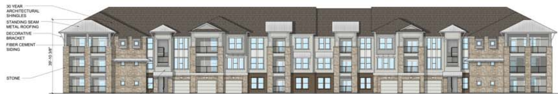
01 BUILDING B FRONT ELEVATION 1/16" = 1'-0"
