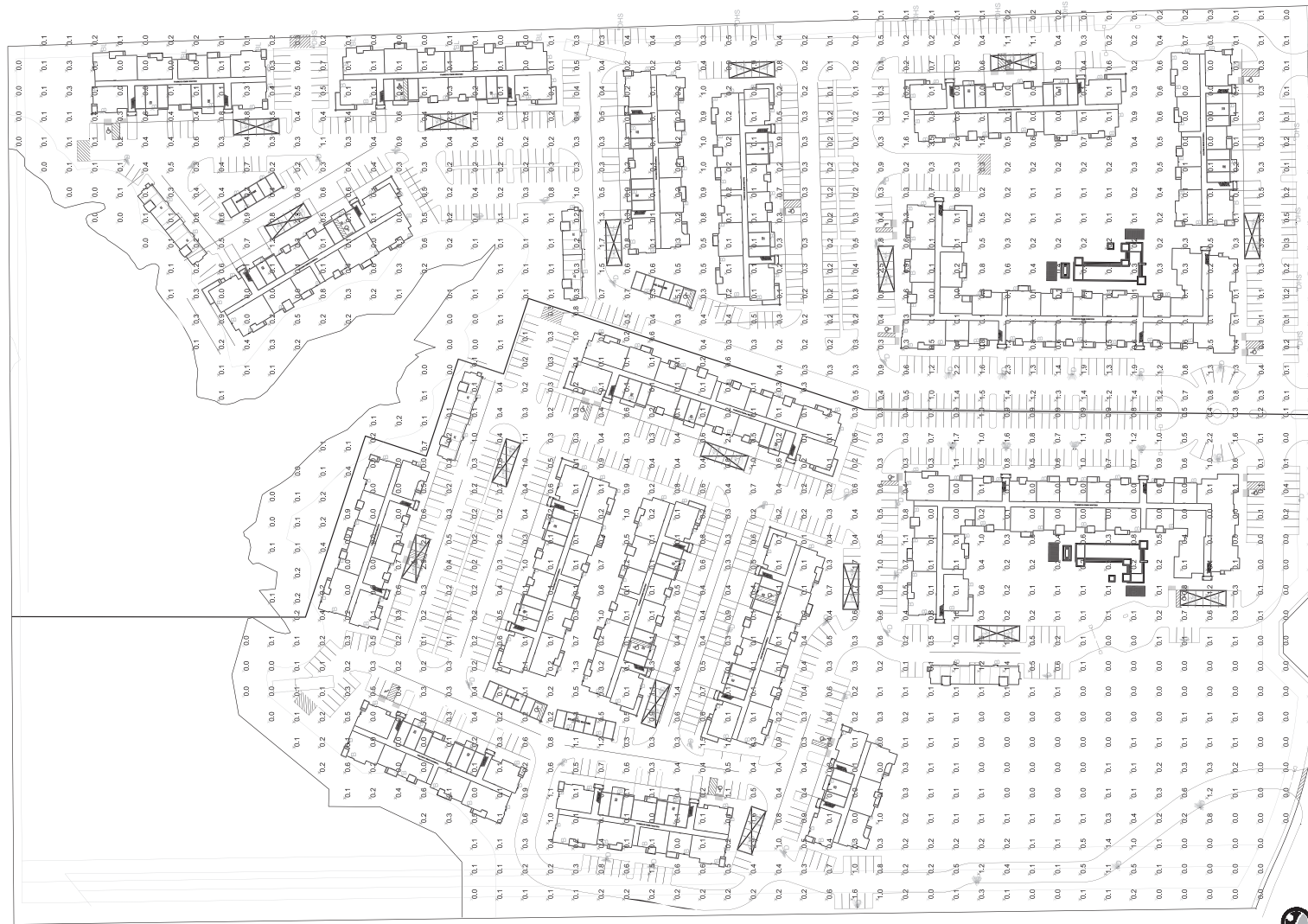
01 SITE PLAN - PHOTOMETRICS SCALE: 1" = 60' 0"
