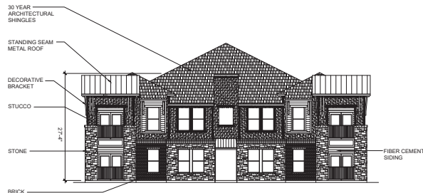
03 BUILDING F SIDE ELEVATION 3/32" = 1'-0"
