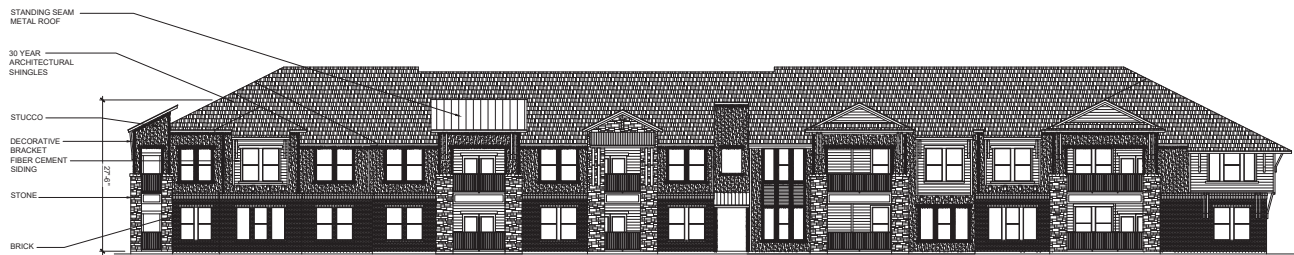
04 BUILDING F REAR ELEVATION 3/32" = 1'-0"
