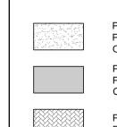
PAVEMENT WITH #3 BARS AT 18" O.C.E.W. PROPOSED 3,600 PSI 5" CONCRETE
