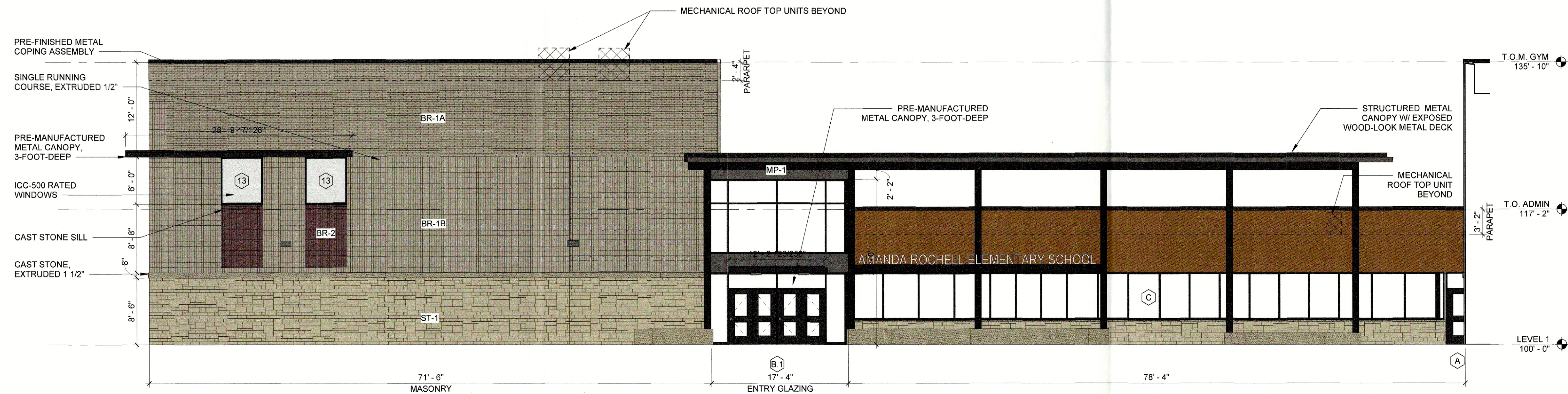
01 EXTERIOR ELEVATION - AREA A - SOUTHEAST 1/8" = 1'-0"
